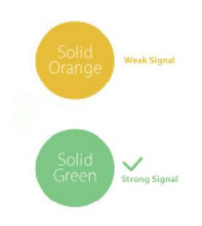
Signal Indicator helps to find the most accurate location to place the range extender
