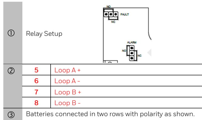
Fig. 16: LT-159 setup and connections overview
