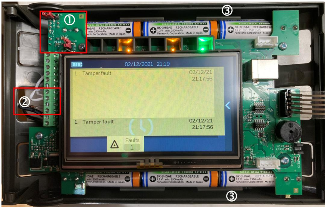
Fig. 15: LT-32 setup and connections overview
