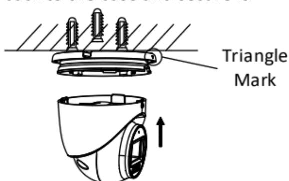
Figure 2-8 Install the Camera Back
