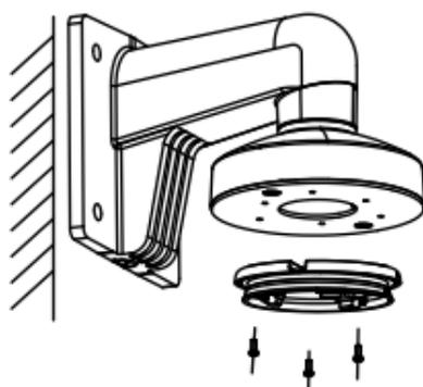
Figure 2-16 Fix the Base onto the Wall Mount
