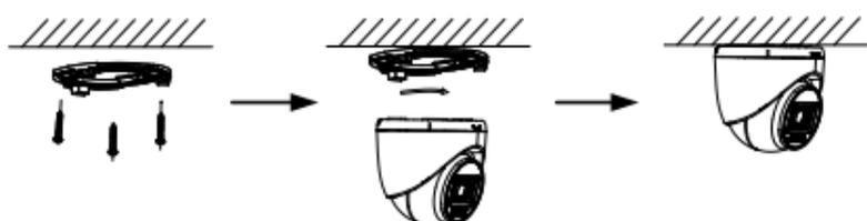
Figure 2-18 Install the Camera to Ceiling
