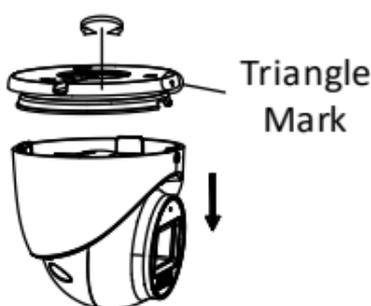
Figure 2-6 Disassemble the Camera
