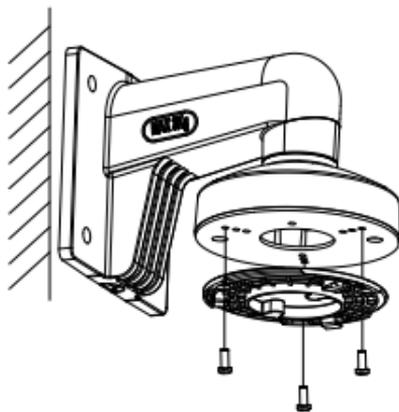
Figure 2-23 Fix the Installation Plate
