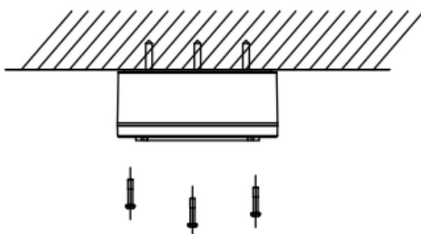
Figure 2-11 Combine the Junction Box Cover and Body
