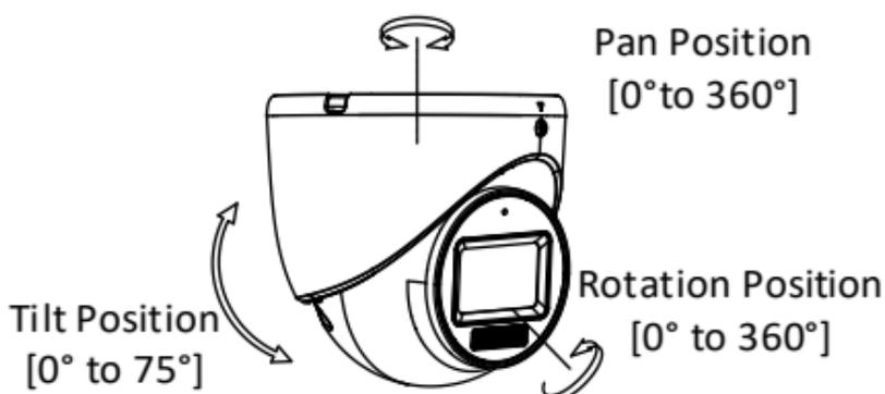
Figure 2-9 3-Axis Adjustment
