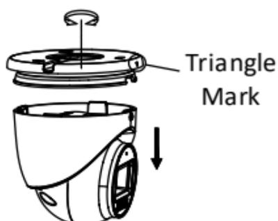
Figure 2-15 Disassemble the Camera
