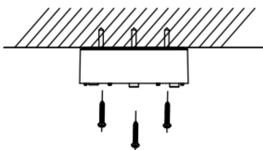
Figure 2-10 Secure the Junction Box Body
