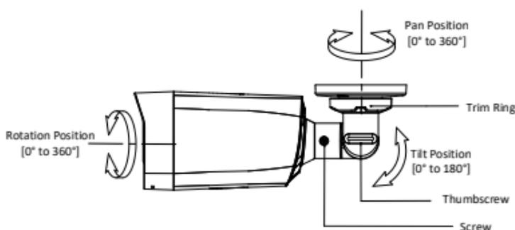
Figure 2-2 3-Axis Adjustment
