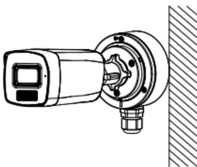
Figure 2-5 Fix the Cover to Its Body
