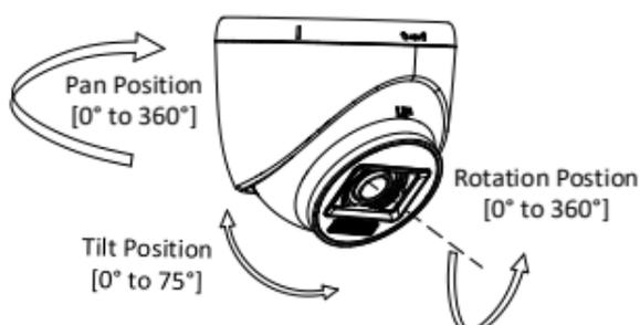
Figure 2-19 3-Axis Adjustment
