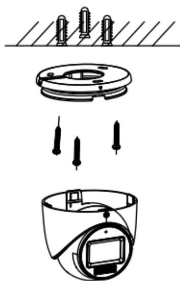
Figure 2-7 Secure the Base to the Ceiling
