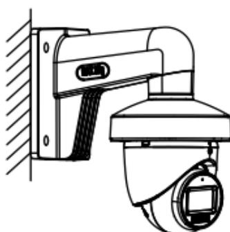
Figure 2-17 Finish the Installation
