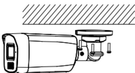
Figure 2-1 Secure the Camera to the Ceiling
